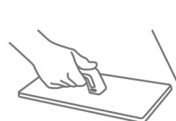
COMPRESSING THE TILE
